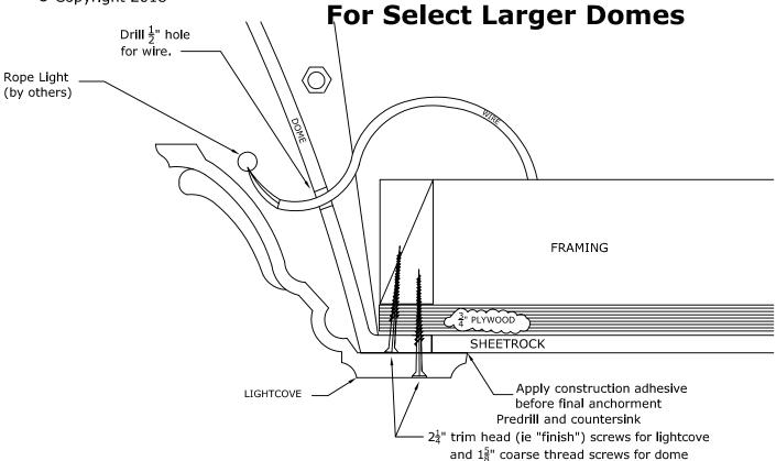
We recommend a minimum of one point of anchor every 16" on lightcove. This is in addition to a minimum of one point of anchor every 16" for the dome bottom flange, and the recommended minimum of tiewire attachments for the dome.
