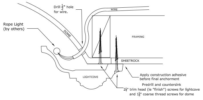
We recommend at least 8 points of anchor for the light cove (in addition to at least 8 points of anchor for the dome). Larger domes may have special framing suggestions.
