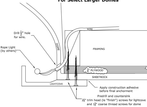
We recommend a minimum of one point of anchor every 16" on lightcove. This is in addition to a minimum of one point of anchor every 16" for the dome bottom flange, and the recommended minimum of tiewire attachments for the dome. Check the spec sheet for your dome.
