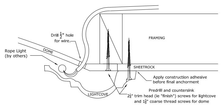
We recommend at least 8 points of anchor for the light cove (in addition to at least 8 points of anchor for the dome).
