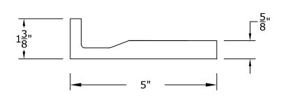
We recommend at least 8 points of anchor for the light cove (in addition to at least 8 points of anchor for the dome). Larger domes may have special framing suggestions.
