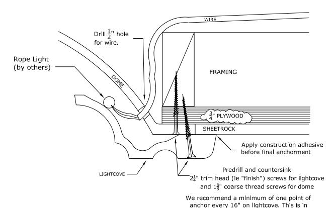
recommended minimum of tiewire attachments for the dome. Check the spec sheet for your 3"
