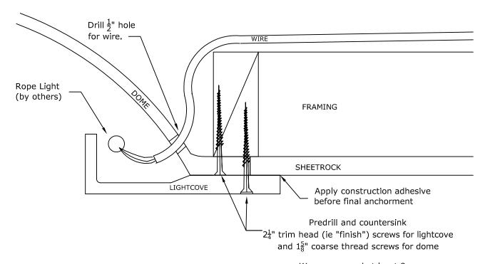
We recommend at least 8 points of anchor for the light cove (in addition to at least 8 points of anchor for the dome). Larger domes may have special framing suggestions.
