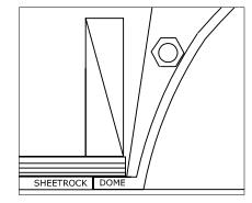
Drill through both bolt flanges for permanent #9 tiewire anchorment (we recommend a minimum of two per flange)
