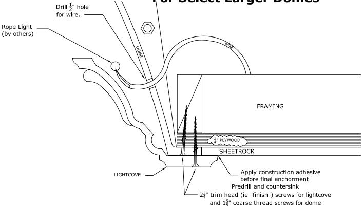
We recommend a minimum of one point of anchor every 16" on lightcove. This is in addition to a minimum of one point of anchor every 16" for the dome bottom flange, and the recommended minimum of tiewire attachments for the dome.
