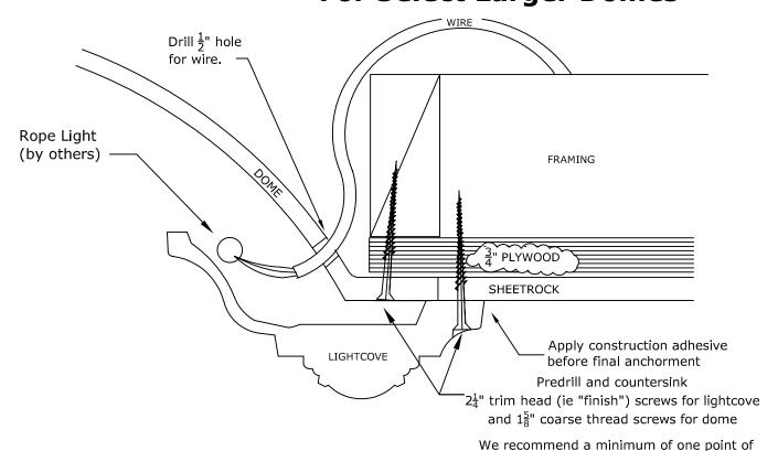
recommended minimum of tiewire attachments for the dome. Check the spec sheet for your LIGHTCOVE
