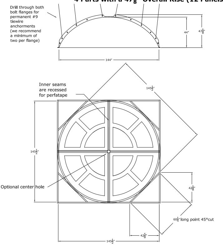
Note: We also add heavy duty loop strapping to the back of the dome for temporary tiewire attachment.
