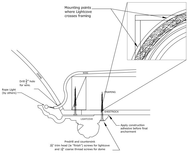
We recommend at least 8 points of anchor for the light cove (in addition to at least 8 points of anchor for the dome).
