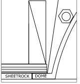
108" Heavy-duty loop strapping cast into back of dome for temporary attachment (i.e. lifting dome as Inner seams one piece) and/or permanent are recessed  $109\frac{1}{5}$ " anchorment (i.e additional for perfatape seismic support). 109<del>1</del>" Optional center hole  $\Diamond$  $\Diamond$ 32<u>1</u>"  $45\frac{3}{8}$ " Long point, cut at 45° 32<u>1</u>" 109号"
