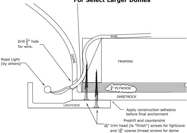
We recommend a minimum of one point of anchor every 16" on lightcove. This is in addition to a minimum of one point of anchor every 16" for the dome bottom flange, and the recommended minimum of tiewire attachments for the dome. Check the spec sheet for your dome.
