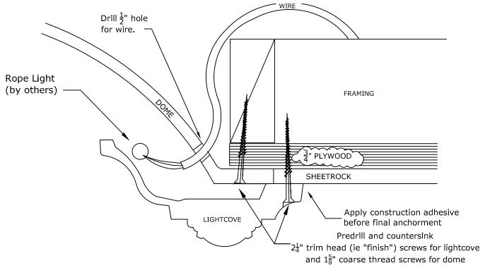
We recommend a minimum of one point of anchor every 16" on lightcove. This is in addition to a minimum of one point of anchor every 16" for the dome bottom flange, and the recommended minimum of tiewire attachments for the dome. Check the spec sheet for your dome.
