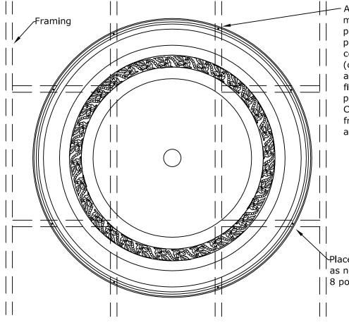
After you have marked all mounting points and a reference point to realign the dome to, predrill (1/8" bit) and countersink (1/4" bit), apply glue (construction adhesive) to flange, and mount to ceiling using 2-1/4" finish screws at all 8 framing points.
